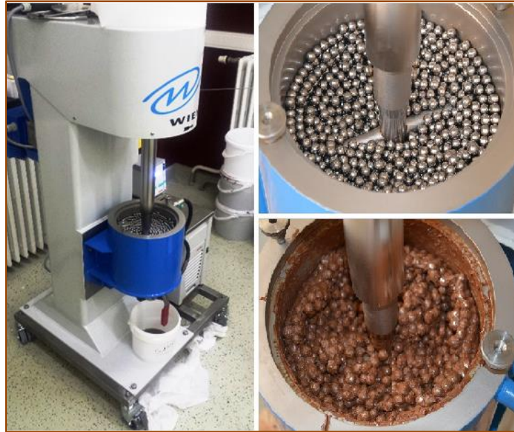
Figure 1.4. Typical ball mill used in the alternative processing (Laboratory scale)
