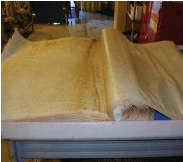
Figure 2. Whole leaf view showing foulants. Courtesy of Protecno s.r.l. Italy.
