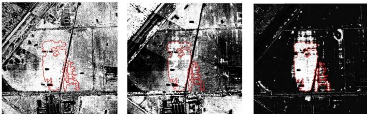
Fig. 7 Comparison of different classification methods: maximum likelihood (left), minimum distance (middle), artificial neural network (right). White colour indicates inland excess waters, all other areas are in black. The training data is shown with a red-coloured boundary
