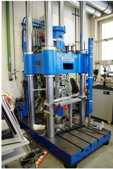
7.14.1: Schenck 400 kN. The Schenck 1000 kN appears identical.
