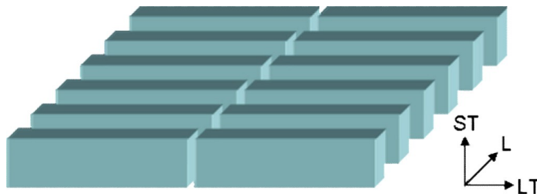
Figure 7.2: Lamination directions in the specimens.
