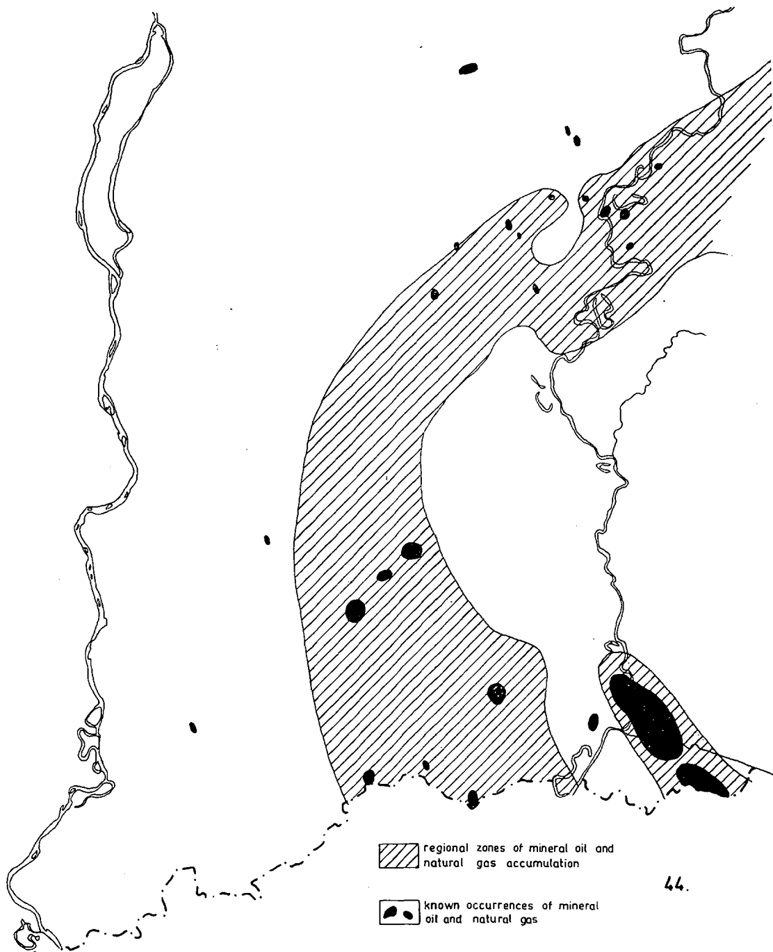
Fig. 44. Known areas of hydrocarbon occurrence between the Danube and the Tisza (KÖRÖSSY—FEHÉR)
