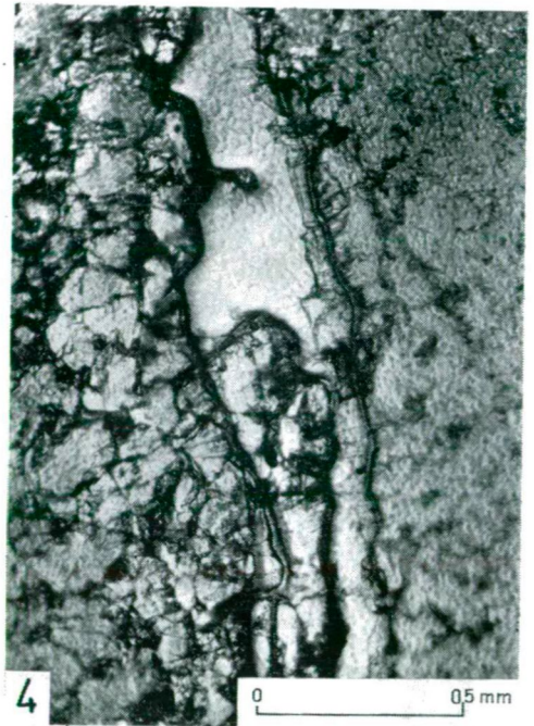
Photographs 1—2. Microphotographs of a hydrothermally cemented dolomite from the vicinity of Pí-lisszentlélek Photographs 3—4. Microphotographs of a hydrothermally decomposed dolomite from the Nagyszál at Vác
