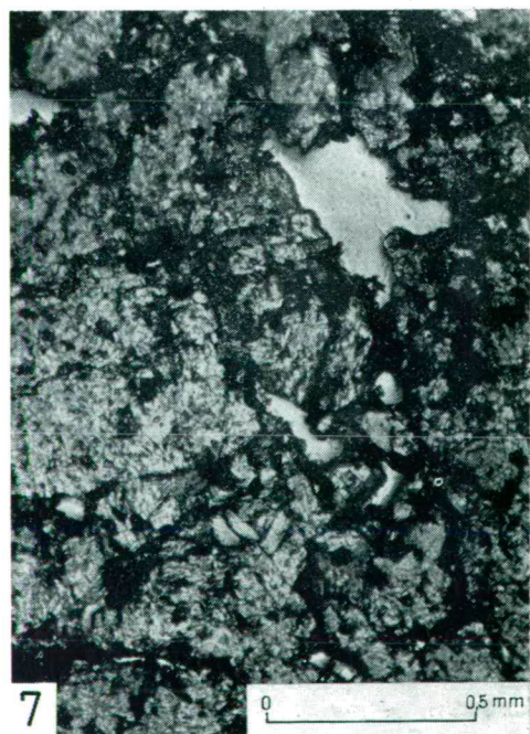
Photographs 5—6. Microphotographs of a calcitized dolomite from the vicinity of Pilisszentlélek Photographs 7—8. Microphotographs of a dolomite of very low magnesite content from the vicinity of Pilisszentlélek
