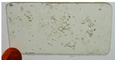
Figure 5.5. Picture of a processed poly(cycloacetal) from glutaraldehyde and di-TMP obtained via protocol A.
