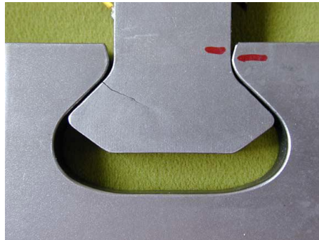
Figure 3.2 Failed blade specimen [Nowell, Dini & Hills, 2006]
