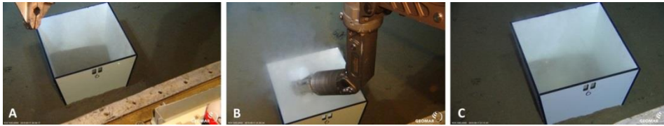
Figure 7.1 Impressions of the deployment of the experimental corrals to test toxic sediment plume impacts on an abyssal meiofauna community, A) prior to, B) during and C) after sediment deposition. Copyright: ROV Kiel 6000 Team/GEOMAR Kiel
