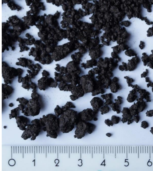
Figure S5.2 Sample of the crushed nodule substrate. Scale in centimetres.
