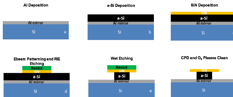
Fig. 5. Schematics of the fabrication flow. (a) Deposition of 50 nm Aluminum layer on top of the silicon substrate. Thin layer of Aluminum oxide (5 nm) and silicon oxide (5 nm) are later deposited on the Al layer to protect the Al layer from oxidation and wet etching. (b) 950 nm of a-Si is deposited on top of Al layer. (c) 220 nm of SiN is deposited on top of a-Si layer as the waveguide layer. (d) E-beam is used to pattern the test structure and RIE etching transfers the pattern from e-beam resist to SiN layer. (e) Wet etching is used to undercut the grating and the waveguide. Some a-Si is left to support the pillar, as shown in the figure. (f) CPD process is used to release the structure and oxygen plasma cleaning is used to remove the residual e-beam resist.
