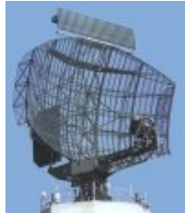
Figure 2.13.SRE-M7, typically en-route radar made by the German DASA company
