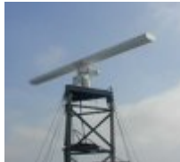
Figure 2.16. Surface Movement Radar ASDE
