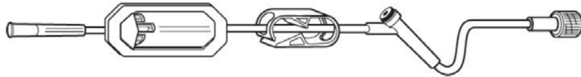
Figura 14 - Non-DEHP Extension Set with 1.2 Micron Downstream Air Eliminating Filter, INTERLINK Y-Site (Baxter Healthcare Corporation).
