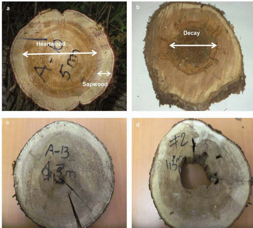
Figure 5.1. Macroscopic structure of heartwood, sapwood, and decay in Thuja occidentalis L.
