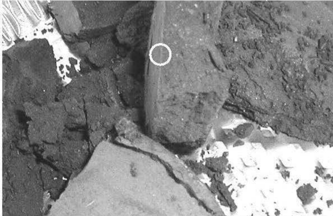
Figure C.13, Pieces of T5-T10/T50 CPB showing a thin desaturated zone (less than 1 mm) at the top.
