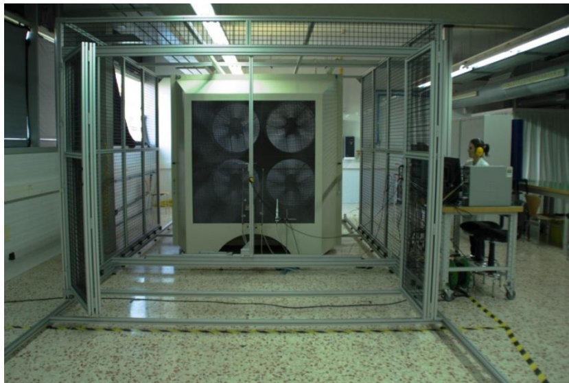
Figure 30: Front view of the 4-Winds Open Jet Wind Tunnel. Instrument carriage and operator's console.
