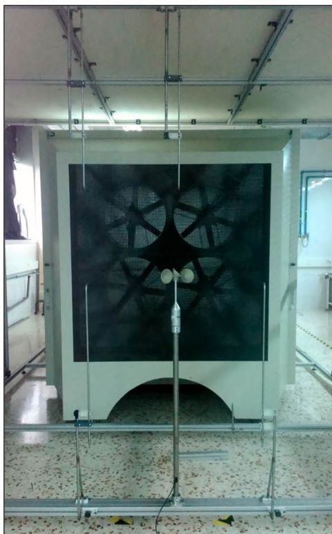
Figure 29: Photograph of the cup anemometer measurement setup.
