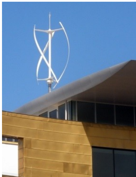
Figure 1: A small Quiet revolution QR5 Gorlov type vertical axis wind turbine in Bristol, England.
