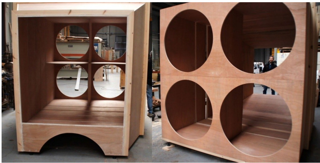
Figure 19: Front and back views of plenum chambers.
