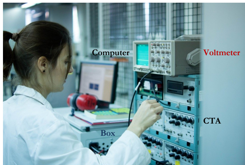
Figure 26: Background, metal box with DPTs and NI CompactDAQ. Foreground, CTA Disa and Voltmeter.
