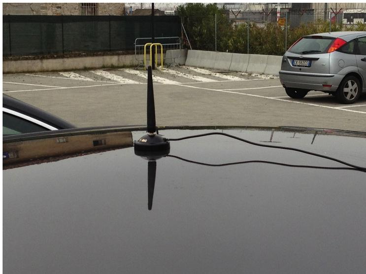
Figura 3.5: Antenna LinkBird-MX
