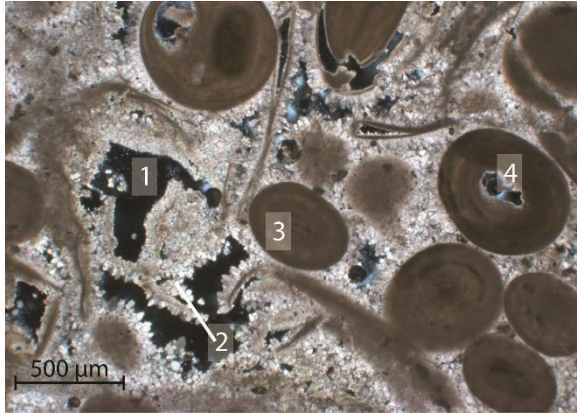
Figure 6.2. Thin section of Savonnières limestone showing intergranular macro-pores (1), intergranular micro-pores (2), intragranular micro-pores (3) and intragranular macro-pores (4).
