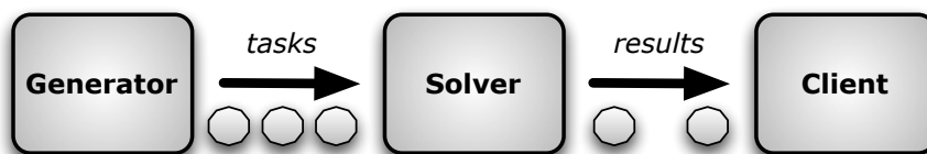
Figure 6.1: Computation graph of the first experiment. In this example the Solver ParMod is the unique parallel module with an adaptation logic.
