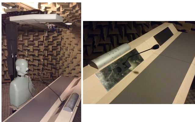
Fig. 3. Automated measurement set-up for the sensitivity comparison between microphone array and goose-neck microphone.
