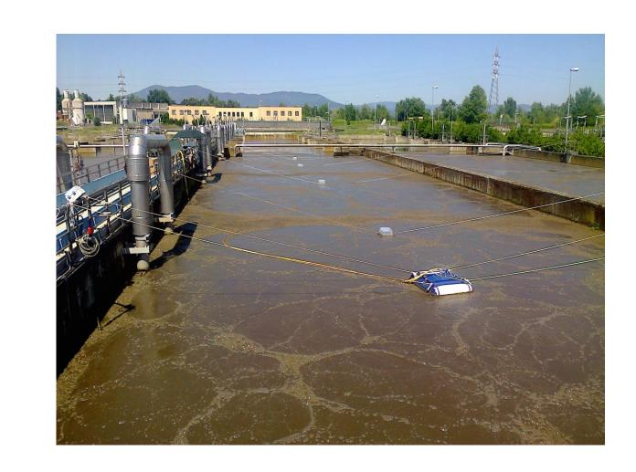
N<sub>2</sub>O was measured with an IR analyzer using 5 hoods in parallel to understand spatial and temporal dynamics and their effect on the emission factor.
