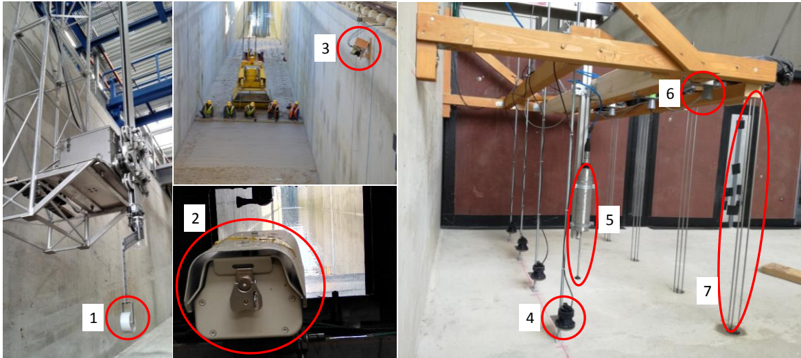
Figure 4. Highlighted in red circles the following measurement devices: (1) mechanical profiler wheel, (2) high speed camera behind observation window, (3) laser scanner, (4) paddle wheel, (5) electro-magnetic current meter, (6) ultrasonic distance sensor, (7) wave gauge on promenade
