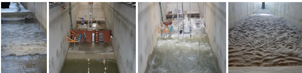
Figure 5. Image of broken wave on foreshore, dry promenade, wet promenade + wave impact, sandy foreshore after approximately 20000 waves (left to right)
