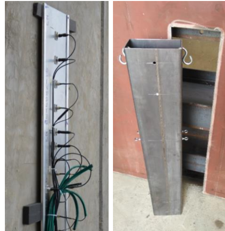
Figure 3. Pressure array (left) and hollow force measurement section (right) before implementation into steel wall
