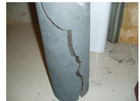
Coil cracking due to differences in thermal expansion rate
