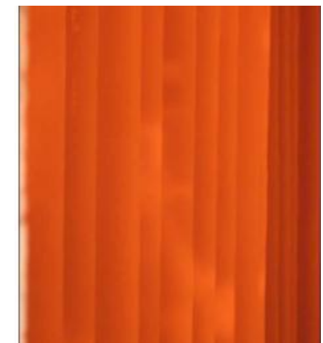
Hot spots due to inhomogeneous coke formation
