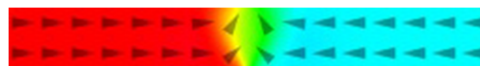
FIG. 8. The transverse domain wall in the center of the nanowire. By compensating the edge charges, we simulate an infinitely long wire.
