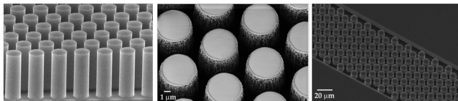
Figure 6.9: SEM images of micropillars etched from a silicon wafer with superficial porosity. Images taken from [261].
