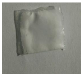
Figure 6.6. A sample of high-purity BaO powder packed into a 2 \times 2 \text{ cm}^2 square PE bag of 0.1 mm thickness. This picture corresponds to the biggest sample size obtained at 660 mg with h = 0.4 + 2(0.1) \text{ mm} = 0.6 \text{ mm} total thickness for irradiations under the channel Cavity. Most samples were \leq 1 \times 1 \text{ cm}^2 and 0.15 to 0.3 mm thick.
