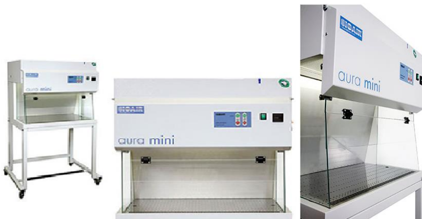
Figure 6.3 The partially recirculating downflow cabinet from LAF Technologies (Australia) model AURA Mini employed in this work for sample drying at room temperature (20 °C) for 24-36 hours. The cabinet complies with a Class 100 (FED STD 209E) - ISO 5 (ISO 14644-1 Standard) environment throughout the work area [193].
