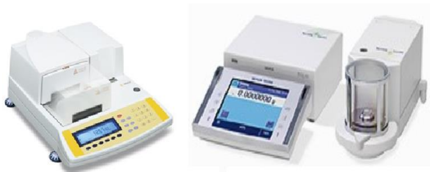
Figure 6.4 The Sartorius Infrared Moisture Analyzer MA100H (left) and the Mettler Toledo XP Ultra-microbalance (right) employed in this work for moisture and sample mass determinations [191, 192].
