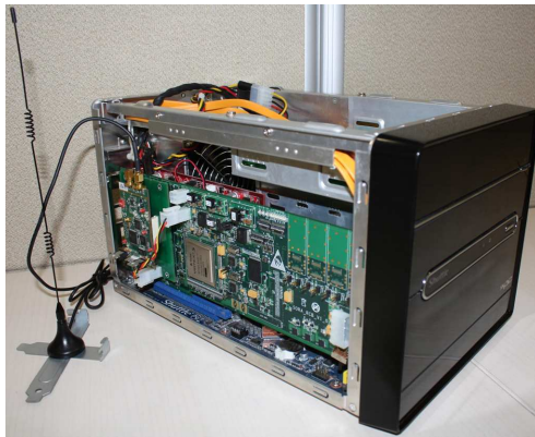
Figure 1.8: Microsoft Research Asia Sora PCIe SDR Board operating within a standard PC
