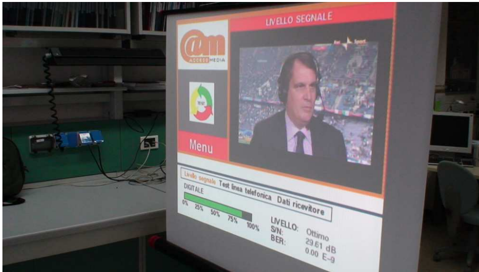
Figure 3.3: Output of the Access Media STB1230 test receiver fed by the Soft-DVB transmitted signal
