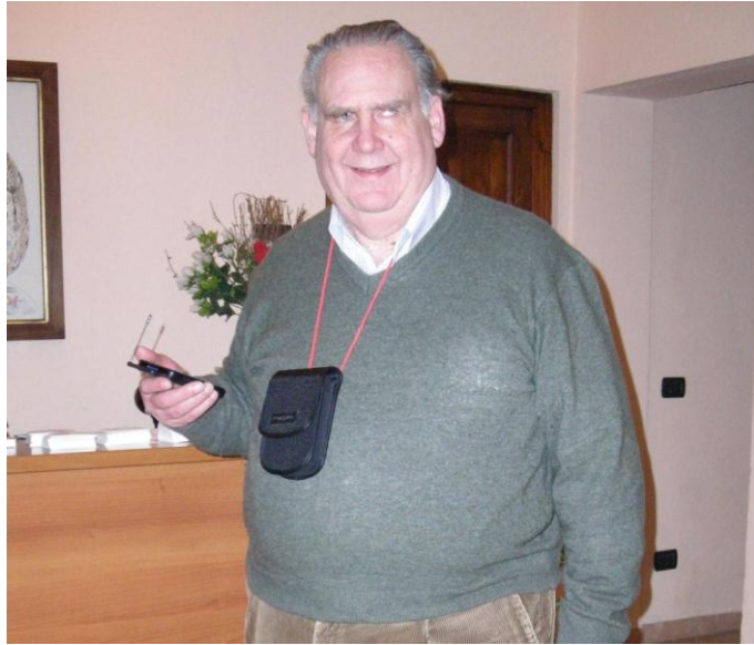
Figure 13: A blind user carrying the early prototype of accessible mobile guide (PDA in the right hand and electronic compass round the neck).
