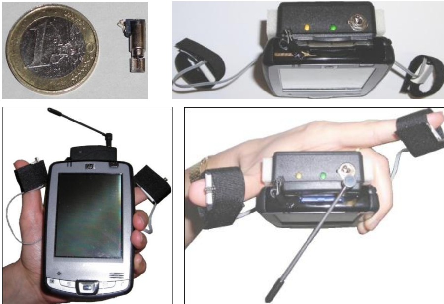
Figure 14. One of the actuators used in the experiment (top left), the PDA fitted with the haptic module (top-right), the mobile equipment fitting on the user's hand (bottom).
