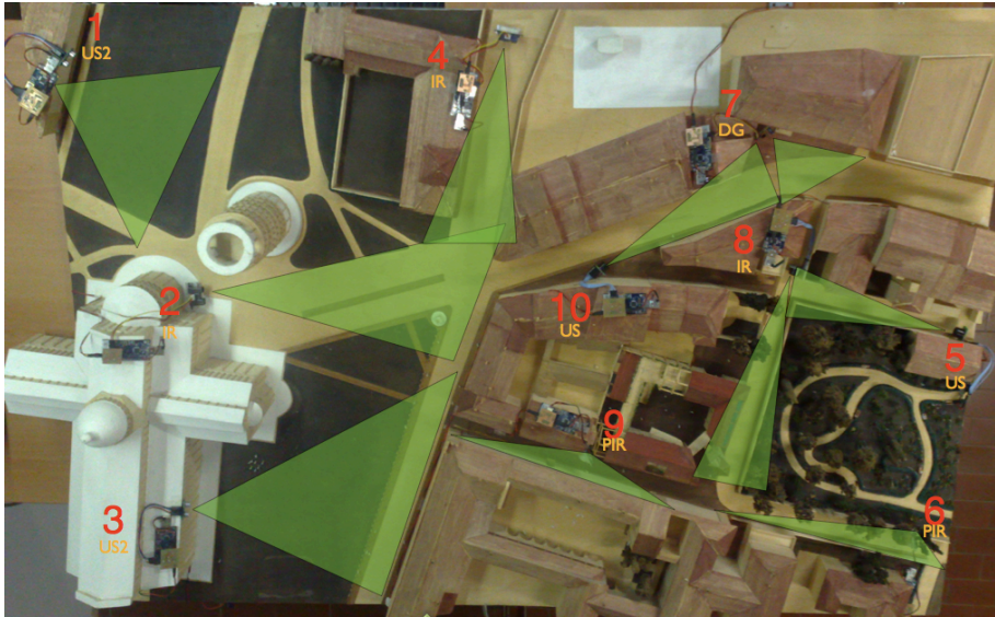
Fig. 5.2 Scale model of the area nearby Pisa's Leaning Tower. Green cones represent the visibility areas of every agents.
