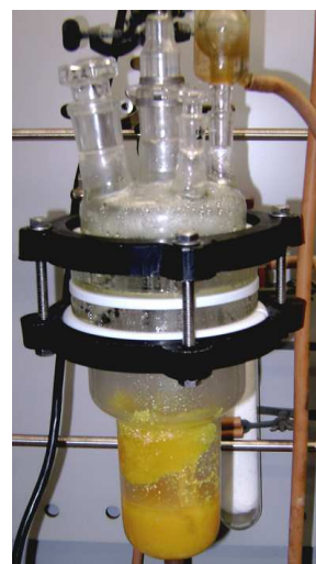
Figure 28. Apparatus for suspension polymerization
