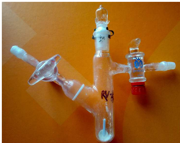
Figure 53. Schlenk tube used for heterogeneous asymmetric transformations.
