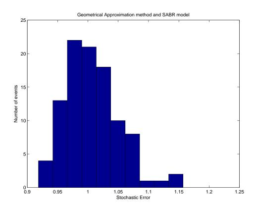
Figure 4.15: Distribution of the stochastic error  $e^{\varepsilon_T}$ , obtained via simulation, for  $\beta = 1$ ,  $\rho = -0.1$ ,  $\sigma_0 = 20\% \ \alpha = 0.29$ , T = 1-year
