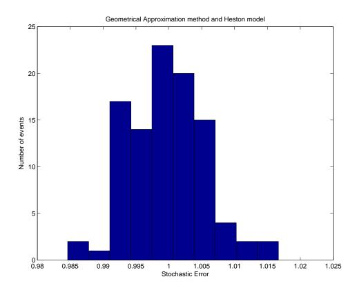
Figure 4.6: Distribution of the stochastic error  $e^{\varepsilon_T}$ , obtained via simulation with parameter values in [6] and  $\rho = -0.1$ , T = 1-month
