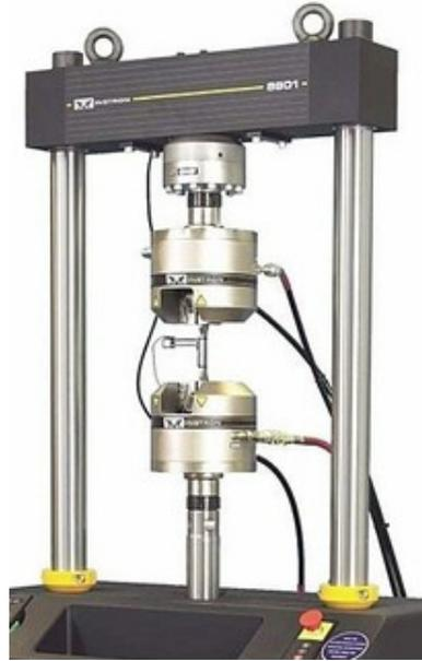
Figura 3.5: *Servo-hydraulic UTM*
