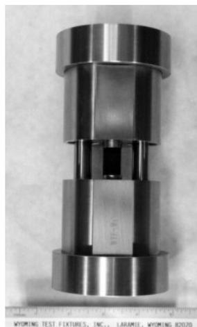
(b) *Wyoming-modified Celanese*Figura 2.7: *Compression fixtures*
