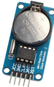
Gambar 9.4: Modul Real Time Clock (RTC)
