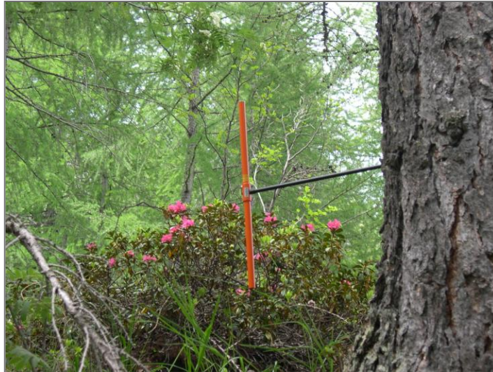
Fig. 3-5 An increment borer in a larch stem
