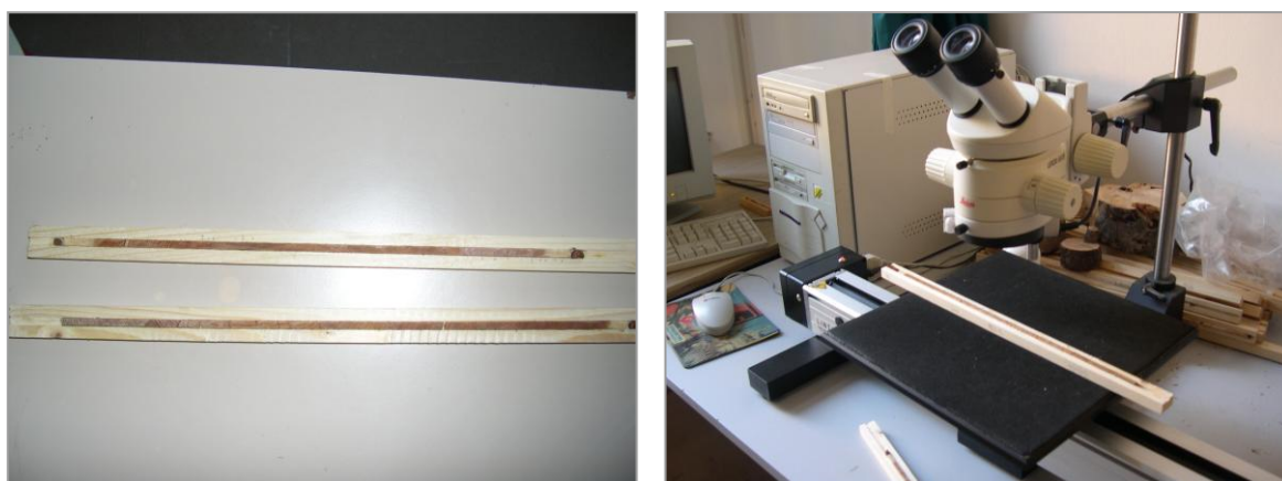
Fig. 3-15 cores mounted on wooden supports ready for measuring and Lintab increment measuring table
