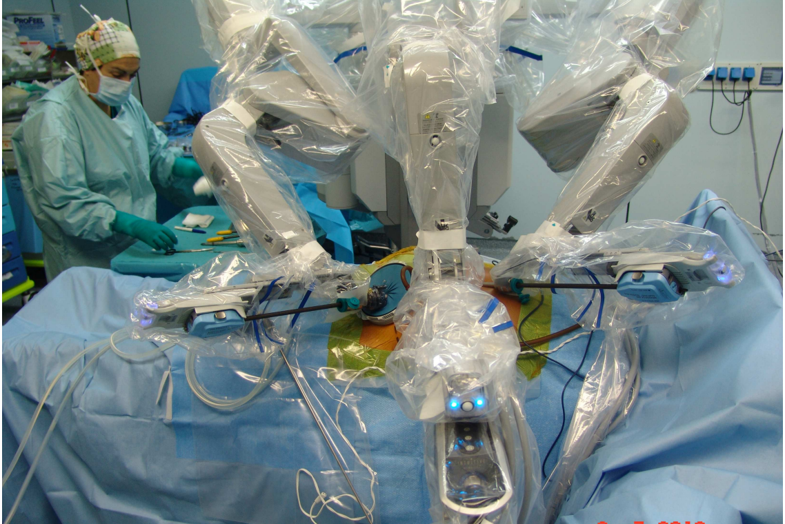
Figure 1c: DaVinci surgical system docked in the operative position.
