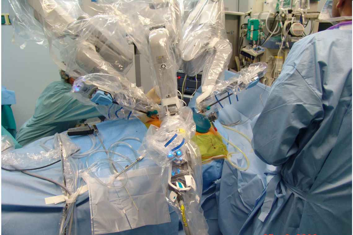
Figure 5: DaVinci Surgical System docked to the operative ports.
