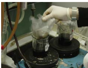
(g) Removal of excess solvent from the sample during regular intervals of weighing
