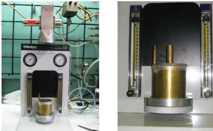
Figure 5.1 Schematic representations for LOI test carried out, (a) LOI equipment without the facility for asphalt, (b) LOI equipment with the facility for asphalt testing
