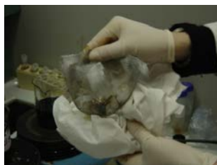
(g) Removal of excess solvent from the sample during regular intervals of weighing
