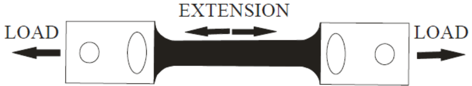
Figure 6.4 Direct Tension Test (DTT)
