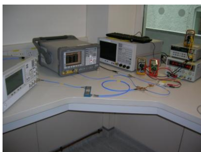
Fig. 23 – Pictures of the NF test setup. Starting from the left: signal generator, spectrum analyzer used as noise figure meter and power supplies on the right.
