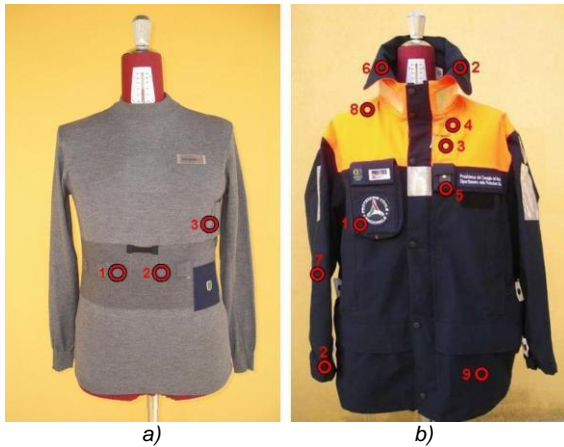
Fig. 5 – Sensor placement on ProeTEX textile platform (a) Inner Garment: 1. Textile Electrodes – Heart Rate monitoring, 2. Piezo-Resistive or Piezo-Electric Sensor – Breathing Rate monitoring, 3. Body Temperature Sensor (b) Outer Garment: 1. Wi-Fi module and Textile Antennas, 2. Wrist & Collar Accelerometers – Activity Assessment, 3. Environmental Temperature Sensor, 4. CO (Carbon Monoxide) Sensor, 5. Visual Alarm Module, 6. Acoustic Alarm Module, 7. Textile Monitor Sensor, 8. GPS receiver, 9. Professional Electronic Box.
