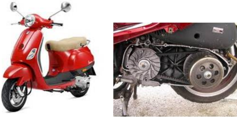
Figure 6.1: Vespa Motor-scooter (left) and CVT assembly (right).
