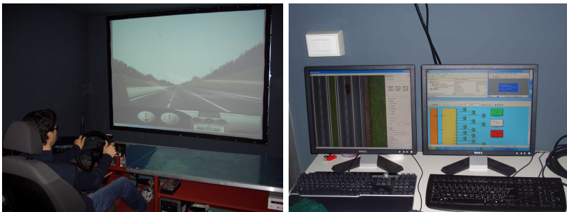
Figure 2.1: Instrumented driving platform (left) and simulator control desk (right).
