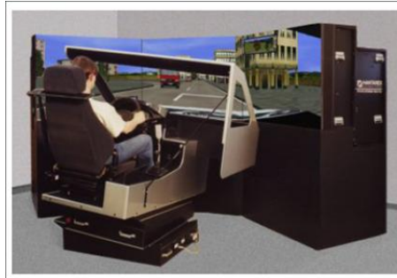
Figure 1.7: Simulator with driver's inputs, one monitor and moving platform.
