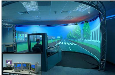
Figure 1.8: Simulator with cylindrical screen and driver's inputs.
