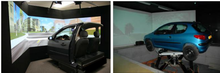
Figure 1.9: Simulators with vehicle and wall screens. On the right, the vehicle is on a moving platform.
