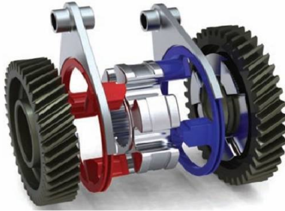
Figure 6.6: Zeroshift transmission elements for a gear pair [25]. The rings are in red and blue.
