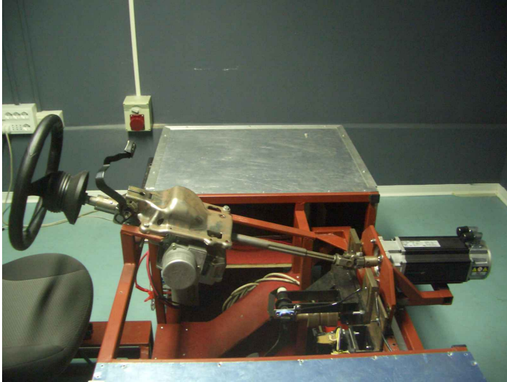
Figure 2.12: Steering system with electric motor for active torque feedback (on the right side of the picture).
