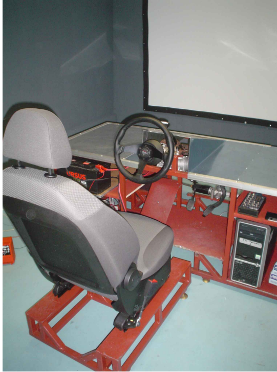
Figure 2.8: Driving platform of the driving simulator.
