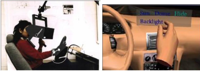
Figure 1.11: Simulator with stereoscopic vision and gloves to reproduce the driver's hands.
