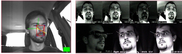
Figure 1.5: Example of eye-tracking system for detecting driver's drowsiness.
