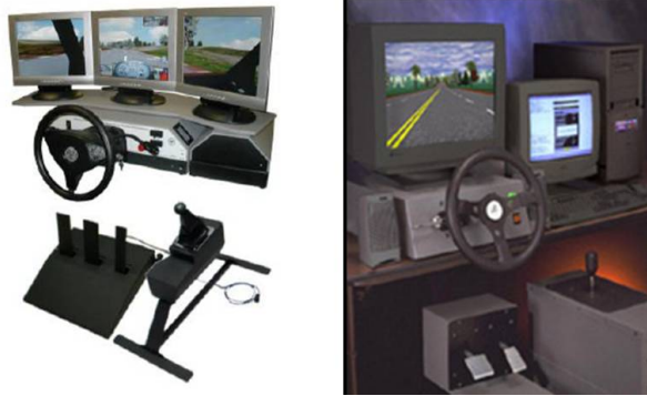
Figure 1.6: Simulator with driver's inputs and three monitor (left) and one monitor (right).
