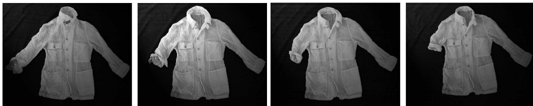
Figure 1.2. Shape-memory-alloy (SMA) integrated into textiles; the sleeves roll up when it becomes too warm.
