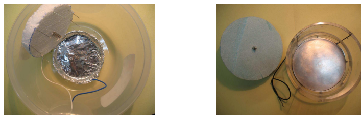
Figure 6.78. Poling cell, first (left) and final (right) version.
