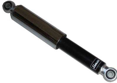
Figure 1.5: A damper used for car suspensions.
