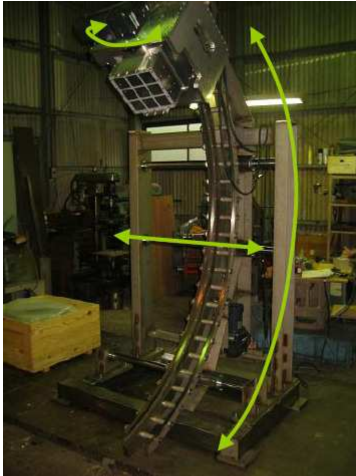
Figure 4.22: NaI detector mounted on a movable mechanical structure.
