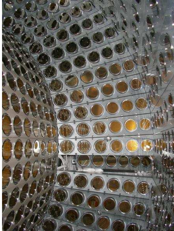
Figure 2.18: Picture of photomultipliers mounted on internal aluminum and peek structure.
