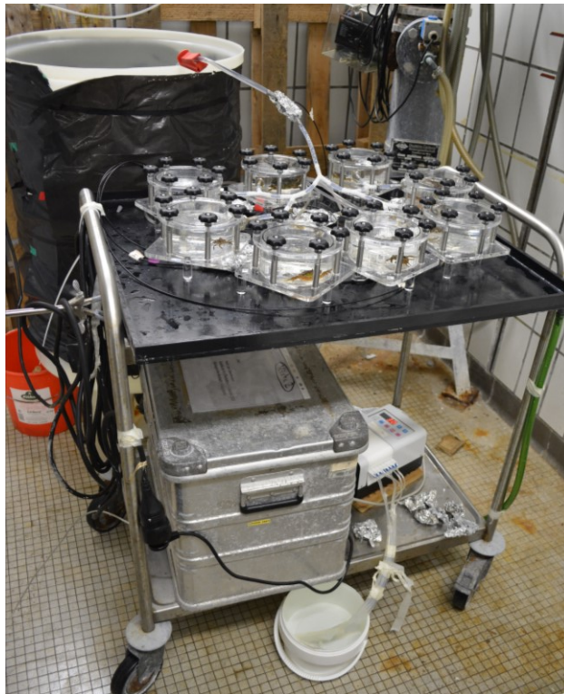
Fig. 2.2: Setup of the respiration measurement device. The water in the tank in the background was pre-tempered in the respective temperature-controlled room. The box on the lower left was holding the actual respiration measuring device, which was connected to the laptop outside in the hallway. Photo: S. Jungblut
