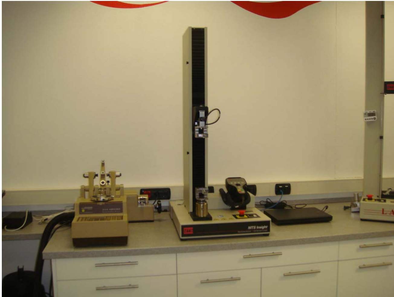
Photo 4. The MTS Insight Dynamometer used for tensile strength tests. September 2009.
