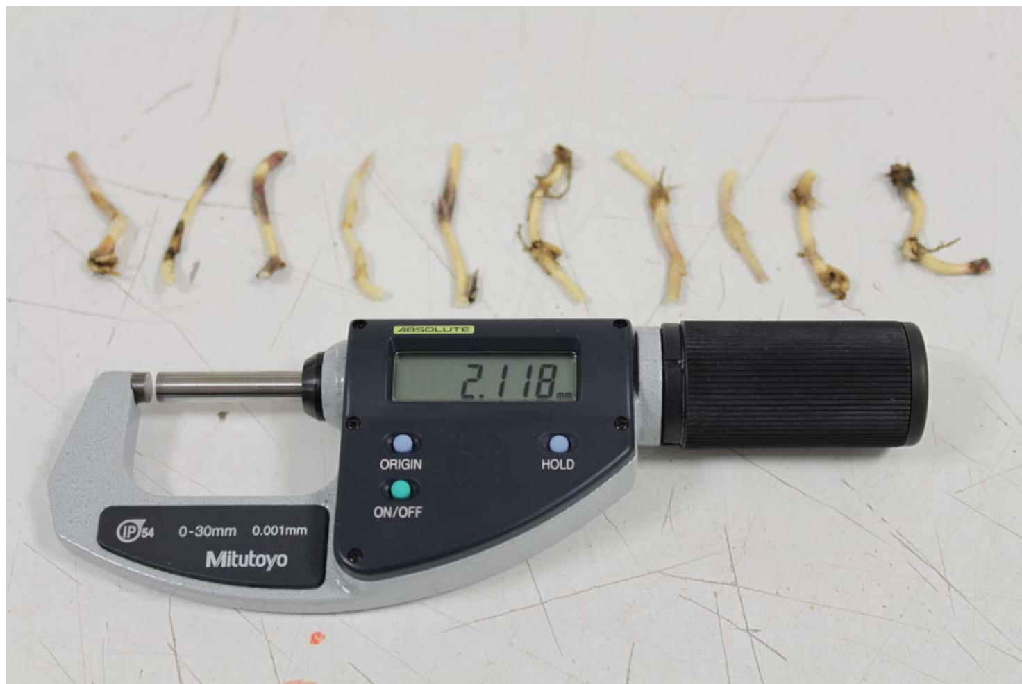
Photo 7. Mitutoyo digital feeler gauge used to measure organ biometrics. September 2009.
