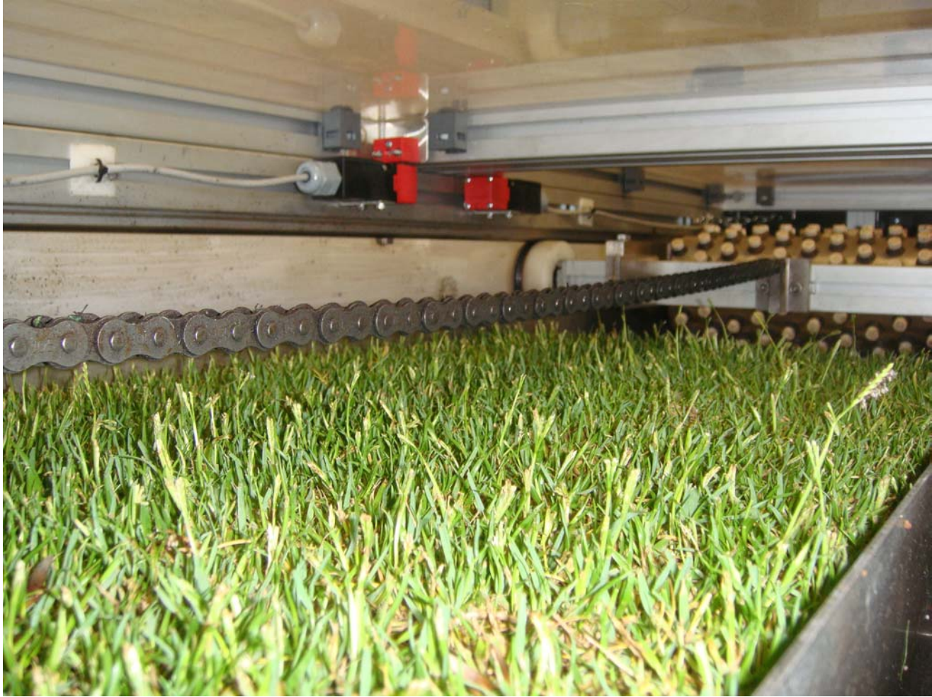
Photo 7. Turfgrass slabs testing in the Lisport machine (2). July 2010.
