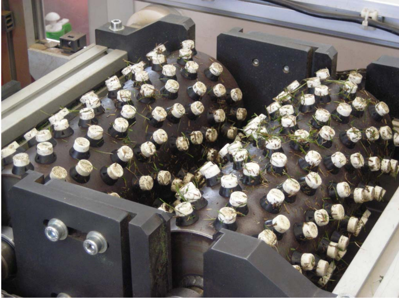
Photo 8. Turfgrass slabs testing in the Lisport machine (3). July 2010.
