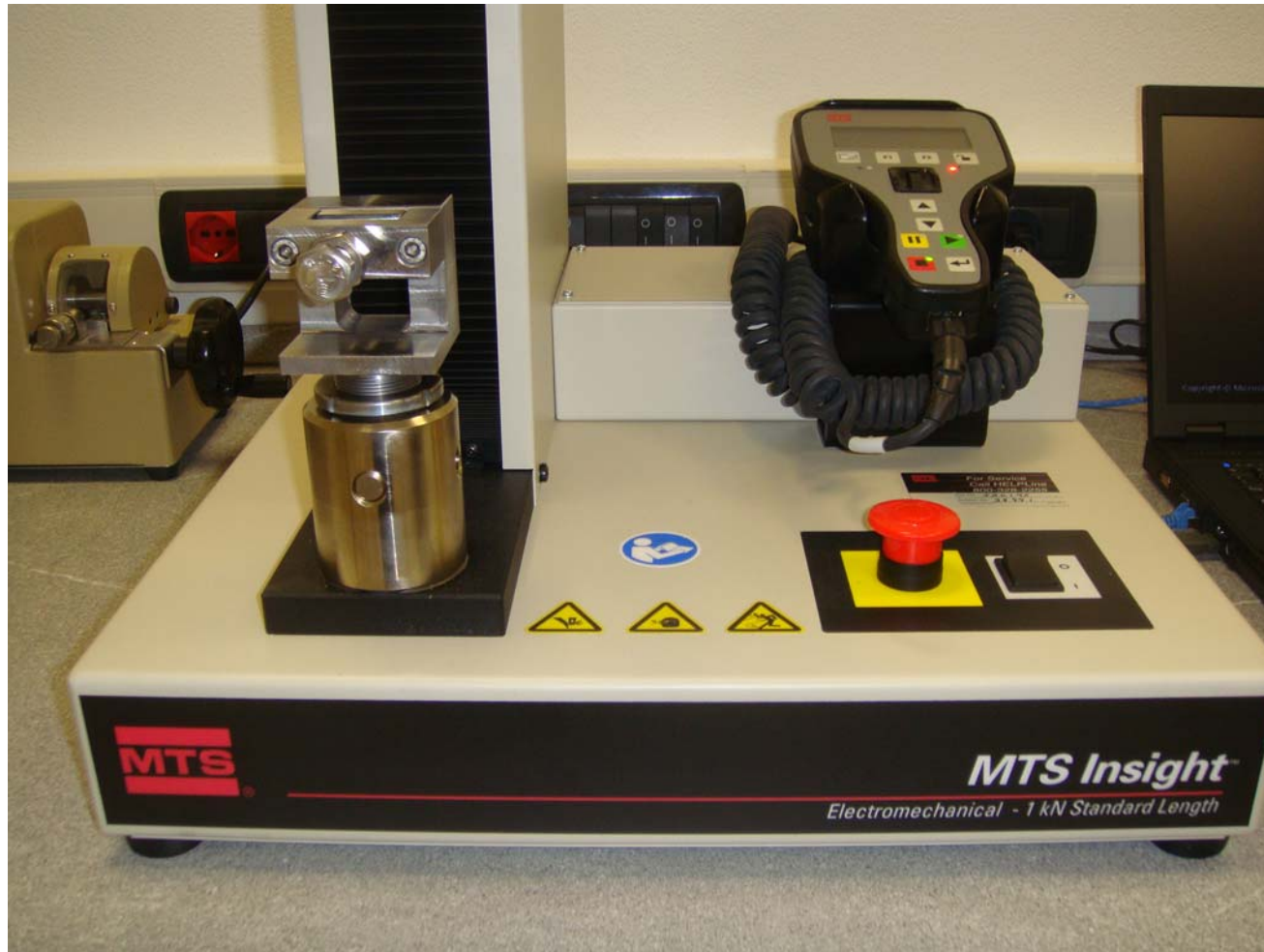
Photo 5. Details of the MTS Insight Dynamometer used for tensile strength tests. September 2009.
