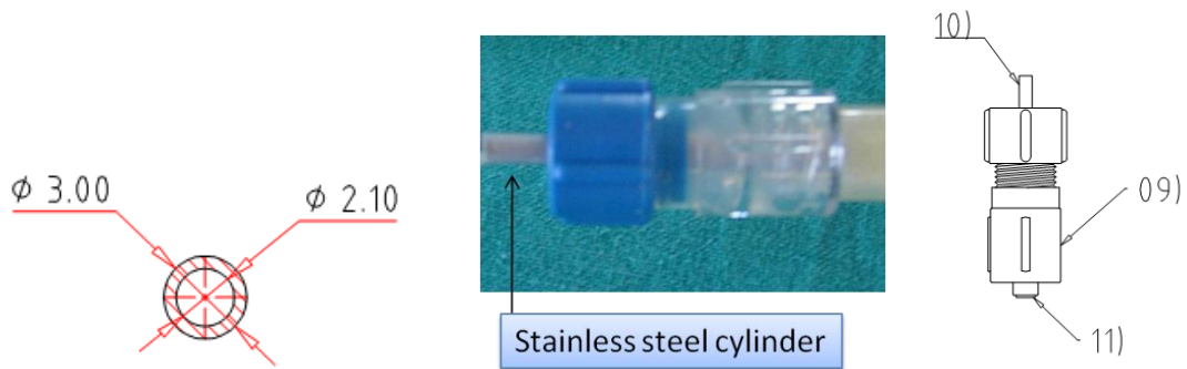
Figure 93 Dimensions the adapter cylinder for the haemostatic valve.
