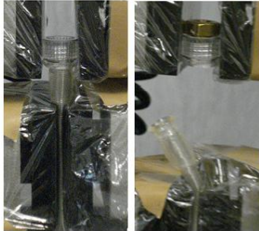
Figure 63 Tensile test on the connection between tube and sleeve
