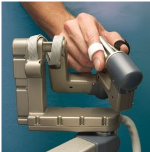
Fig. 2-6 The da Vinci handle used to remotely move the instruments tip.
