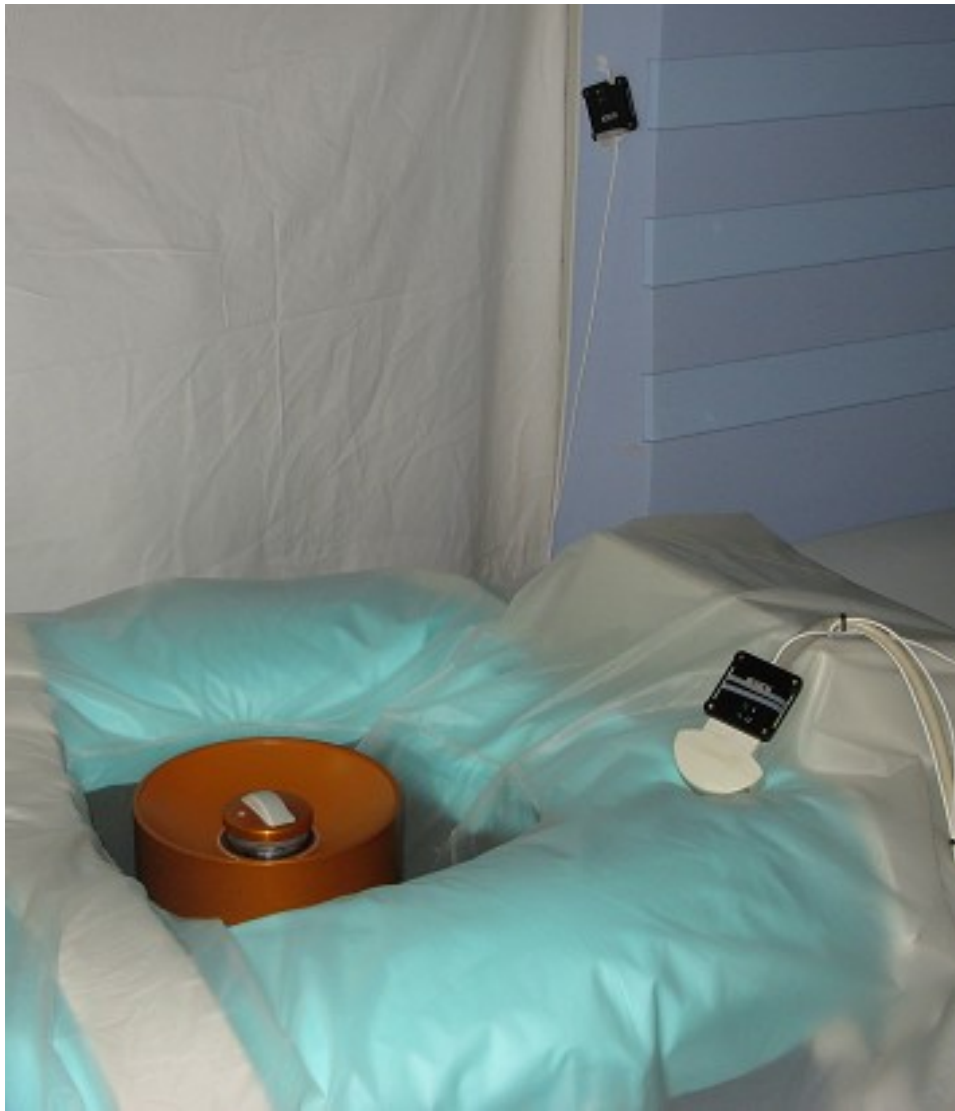
Fig. 5-7 optical sensors fixed on the HIFU machine and ultrasound probe
