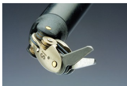
Fig. 2-3 Detail of a microsurgical Endowrist™ instrument: round tip scissors.
