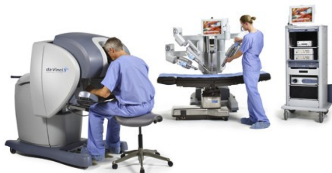
Fig. 2-5 The surgeon at the console and the patient side cart (on the background).
