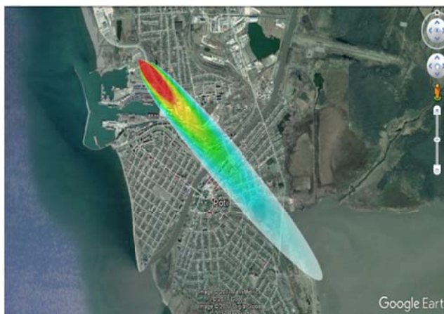
Figure 5 Visualization in ADAM of spatial dispersion of a toxic plume on a local map (Luciano Fabbri, EC-JRC, CARS ADAM Training)
