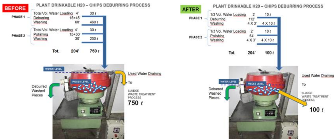
Figure 28: Water use optimisation in deburring
