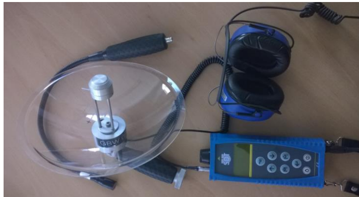
Figure 20: Ultrasonic testing device with rod and parabolic microphone
