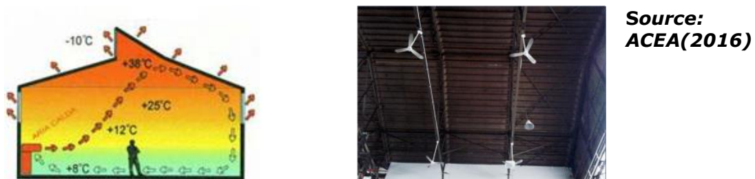
Figure 10: Principle of destratification fans and example installation
