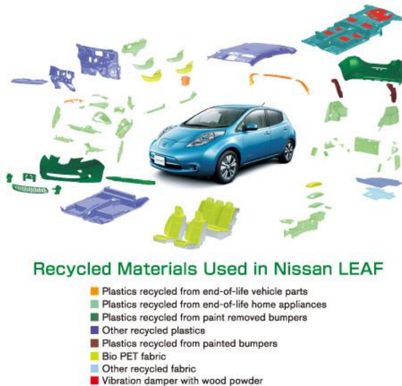
Figure 48: Overview of recycled materials used in the Nissan Leaf
