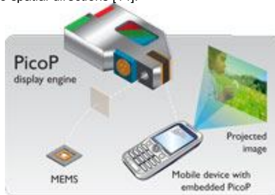
Fig. 16 Example of pico projector integrated in a cell phone (source [15])
