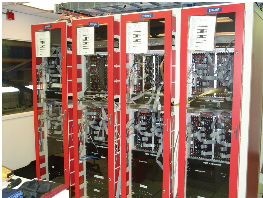
Figure 4.2: The SVT racks - SVT is made by 104 9U VME boards in ten crates. The picture shows the four main racks containing all the system up to the Track Fitting and Final Merge and Corrections that are in other two crates in another rack.
