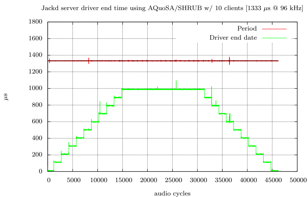
Figure 4.19: JACK perturbed driver end and period with 10 clients, with 2 rt-app tasks running in background using AQuoSA with SHRUB for both JACK and rt-app .
