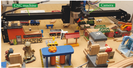
FIGURE 9: Experimental setup showing a camera mounted on a CNC machine allowing us to capture ground truth information. Camera mounted on a CNC machine.
